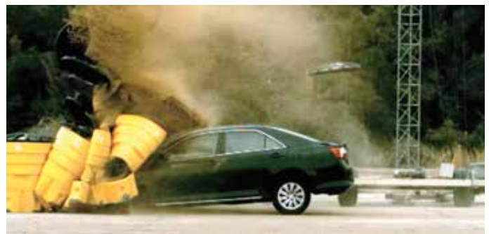
Mash Test Level 3-45, Spring 2018.
