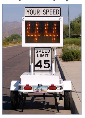
The RU2 Fast-870 Speed Display Trailer has a 18" tall character display and when in full operating position, stands over 8 feet tall. The speed display sign folds down creating a low trailer profile for easy transport and storage. Standard features include high & low speed blanking, flashing digit violator alert and traffic management arrows.
