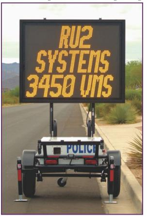
The most versatile Variable Message Radar Sign available, the RU2 Fast-3450 Series Speed Display Trailer has a 40" x 50" full graphic, medium density LED array capable for 1 to 4 lines of text, full graphic characters and complex animation. Whether its speed awareness, a DUI checkpoint, event promotion or traffic management, you can keep the "3450" busy 7 days a week!
