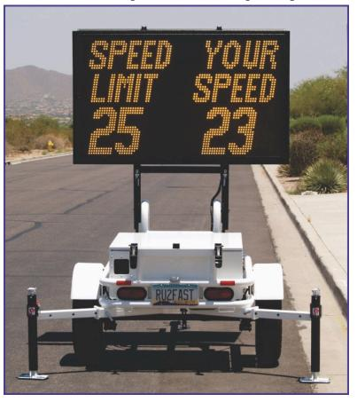
The RU2 Fast-3350 VMS Series Speed Display Trailer has a 30" x 50" full graphic, medium density LED array capable for 1 to 3 lines of text, full graphic characters and complex animation. The VMS display sign folds down creating a lower trailer profile for easy transport and storage. Standard features include high speed blanking, flashing digit violator alert and traffic management arrows, a basic VMS message library and customization software for both text and animation.
