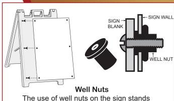
The use of well nuts on the sign stands makes changing signs easier by providing permanent mounting holes
