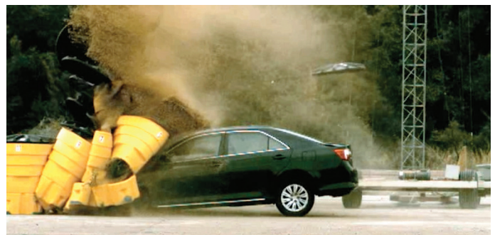
Mash Test Level 3-45, Spring, 2018.
