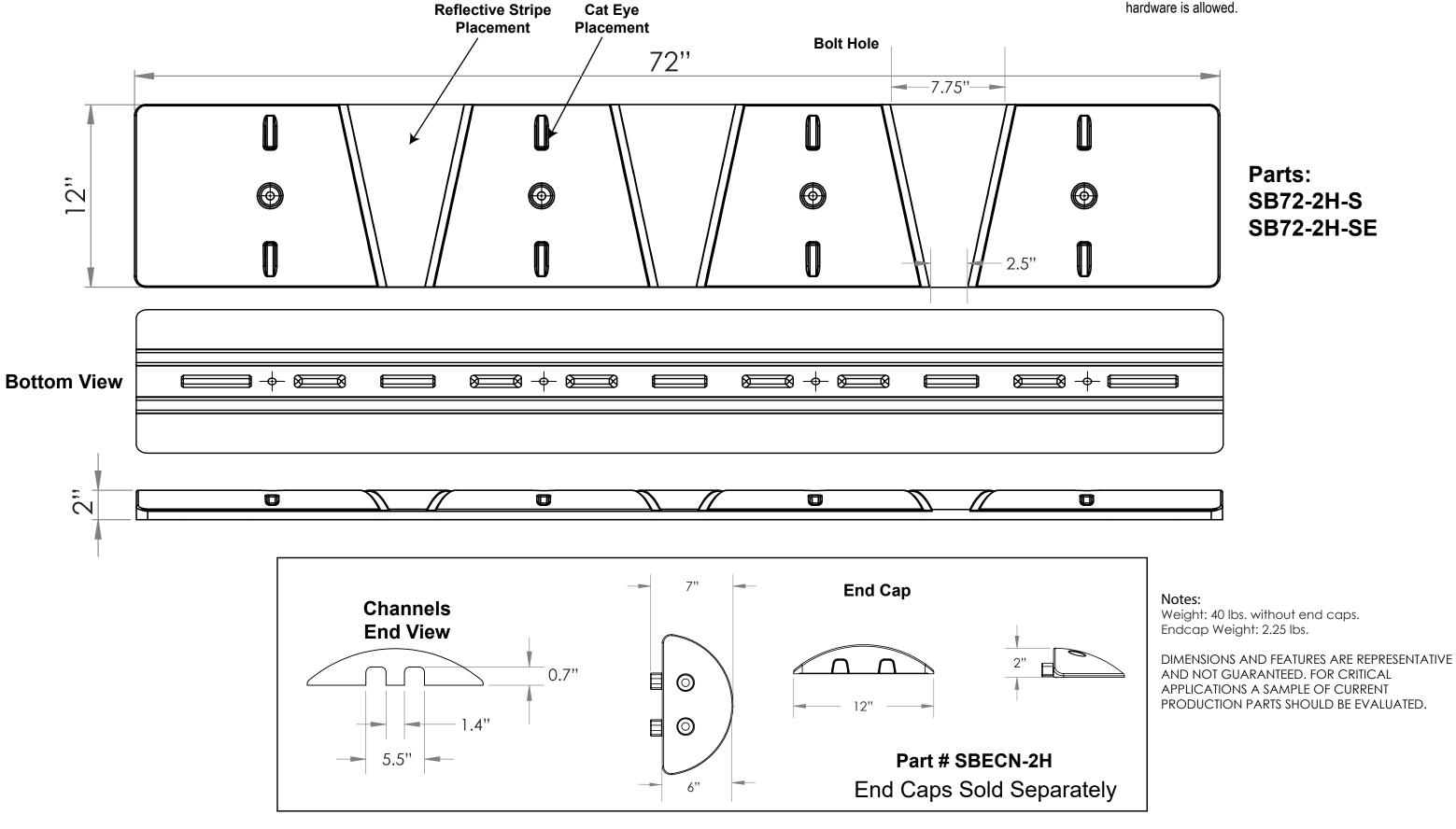
Hardware installation holes are drilled with a  $\frac{1}{2}$ " drill bit. Hardware available:
